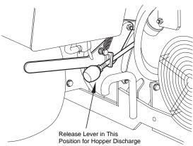
**Figure 4-9 Hopper Operation Position**
